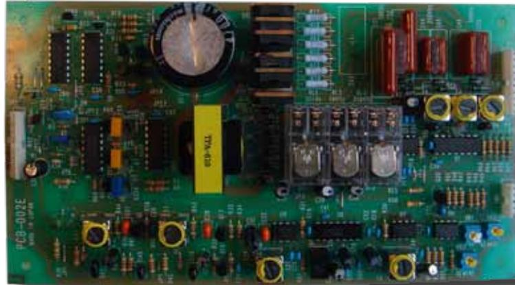
***The PS-G002 is a Calibrated PCB Transceiver for the SKIPPER GDS101 Navigational Echo Sounder.***
